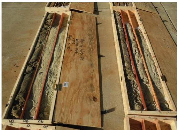
Figure 33: Borehole correlations were made across all of the borings on the Leighton transects to look for vertical separations of key marker units that might confirm the faults shown by PB. Here, there is excellent correlation of the underlying San Pedro contact between borings CB-3 (left) and CB-4 (right) at ~25-30 m, despite being on opposite sides of a mapped fault. The BHUSD team then conducted a similar side by side core comparison of the MTA cores, which encountered and resolved numerous MTA boring log errors.
