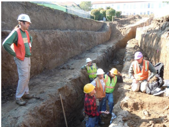
Figure 37: Mixed team peer review of trench FT2 on BHHS campus. Present were representatives of CGS, USGS, and City of Beverly Hills and BHUSD consultants. All trench logging and core comparisons and conclusions were peer reviewed in the field, which also included several MTA consultants at various times. This openness to discuss varying interpretations in front of the physical data led to consensus of interpretation and facilitated the CGS regulatory review.
